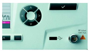
**RF IN/OUT** is a 50  $\Omega$  N-type connector (female) on the right-hand side of the front panel.
