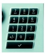
You can open the currently highlighted input field and enter new values or text just by using the entry keys. The Enter key (marked with a tick) is used to accept the current value.
