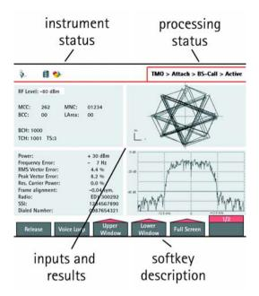
The top row shows the instrument status on the left. This includes the status of battery, network and USB connections.
