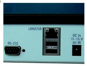
There is an RJ-45 LAN plug on the right-hand side of the rear panel. Additional USB plugs can be found below the LAN plug.
