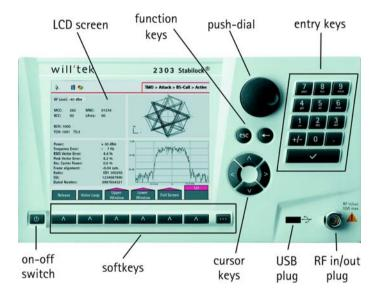
**LCD** The LCD screen shows the menus that guide you through configuration and measurements when the 2303 Stabilock is switched on and the operating software is loaded. The menus consist of four different sections:
