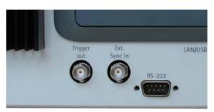
The **EXT. SYNC IN** plug can be found on the rear panel. It can be used as an input for an external time base (reference clock). If an external 5, 10 or 13 MHz clock is connected, the 2303 will automatically use this clock as a frequency reference, and display a symbol on the LCD screen. See the user's guide for more details.
